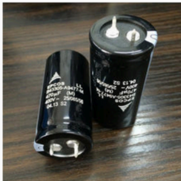
Capacitor 470Mfd/400V Epcos
